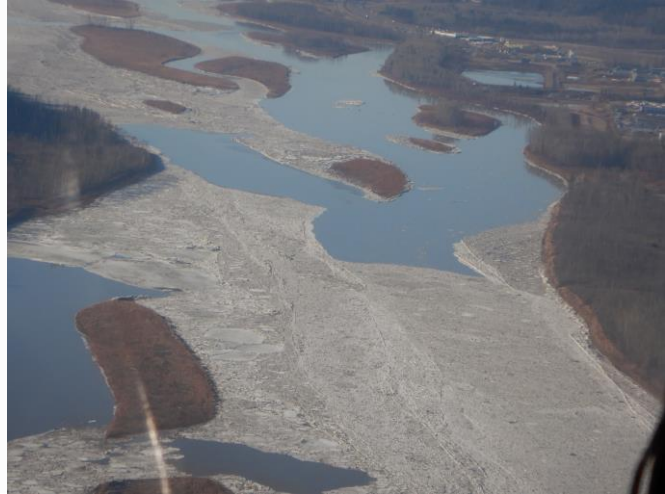
Ice jam head (upstream end) of the 7.3 km long ice jam on the Athabasca River near Fort McMurray. Flow is from top to bottom. Photo taken April 23, 2022 courtesy AEP
