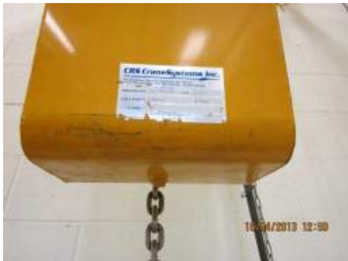
Photo 17: 2 tonne monorail hoist certification has expired according to inspection sticker.
