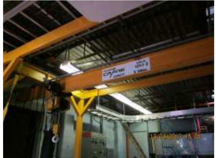
Photo 6: Monorail crane SN 1250-2 on the main floor of the Dry Well. The crane inspection certificate may have expired.
