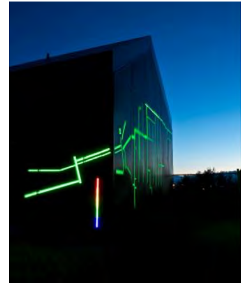
Forest Lawn Lift Station, created by Sans façon. Budget: $236K. In 2015, artists worked with the infrastructure design team to create a map of LED bar lights that are an exact representation to scale of the pipe system in the community. Connected to sensors that monitor the flow of wastewater in the pipes, the lights change colour based on flow levels. Sans façon focused on the process of revealing part of a much larger system.
