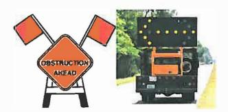
A Moving Operation would utilize A-frame mounted advanced warning signing and a mobile arrow board.
