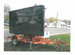
Variable Message Sign boards may be utilized ONLY where conditions change daily or more frequently. Caution must be utilized to ensure the control systems are secure to prevent vandalism and the unauthorized changing of the message.
